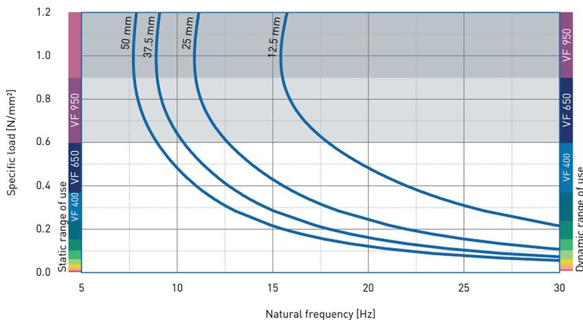
Natural frequency of a single-degree-of-freedom system consisting of a fixed mass and an elastic bearing consisting of VIKAFoam VF 650 on a stiff subgrade.
