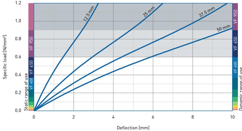
Recording of the 3rd loading; testing between steel plates at room temperature measured with a deflection rate of 1% of the thickness per second
